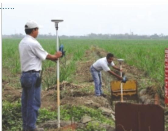
Figure 3 - Obtaining satellite signals with K-GPS receivers to determine the position of corner points of the management units. Note the post with the 6-digit code (091502) of the management unit
